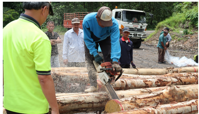
Photo: Cutting a disc sample from the end of the log
