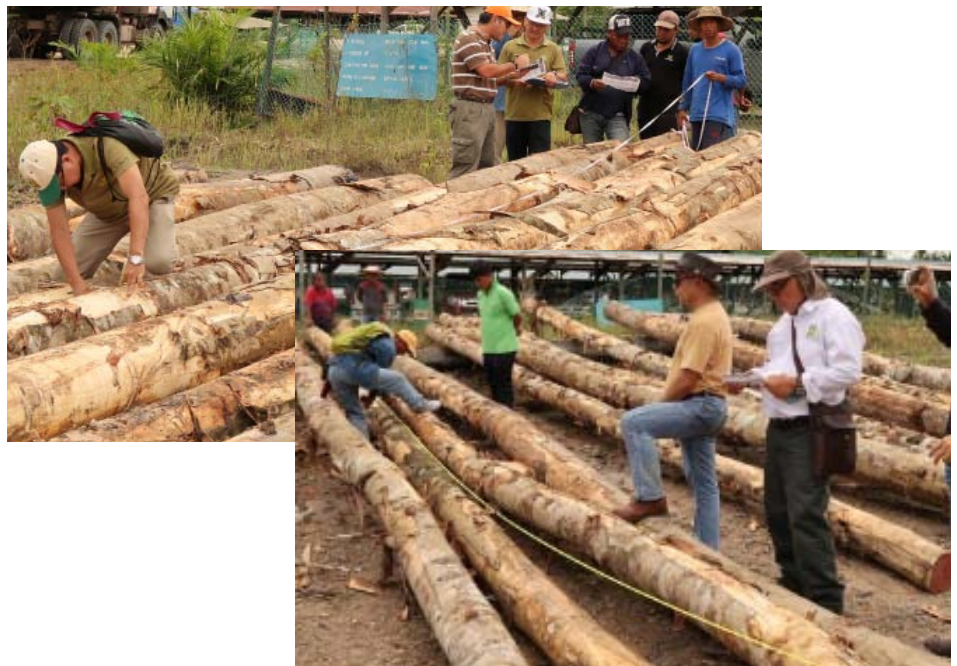
Photo: Research personnel measuring and recording the diameter (top photo) and length (bottom photo) of Albizia falcataria planted logs that were felled.
